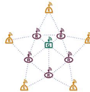
Figure 1: i-Bean Network. (E - Endpoint, R - Repeater, G - Gateway)
